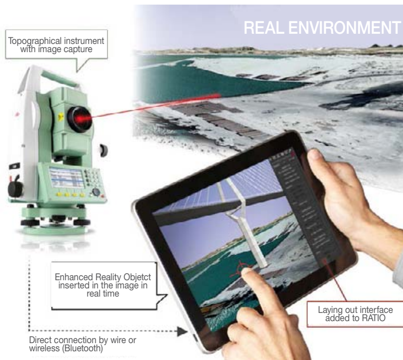
Basic operating schematic of the RATIO system.
